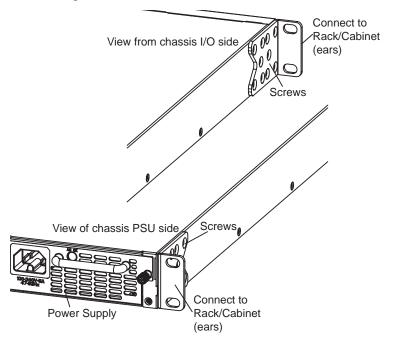
Attach the long bracket to each side of the chassis using the provided countersink screws. Use two screws on each side of the chassis.
