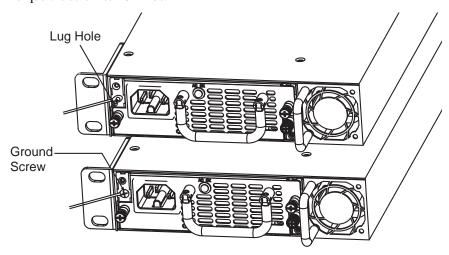
Attach the other end of the ground cable to a suitable ground point. The rack installation ears are not a suitable 4 grounding point.
