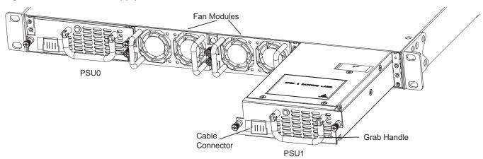
Power supply 0 (PSU0) is on the left side of the chassis; power supply 1 (PSU1) is on the right side of the chassis.
