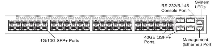
**NOTE:** The SFP+ ports (Figure 2-2) are labeled 0-47. When you cable these ports, be sure not to interfere with the airflow from the small vent holes above and below the ports.
