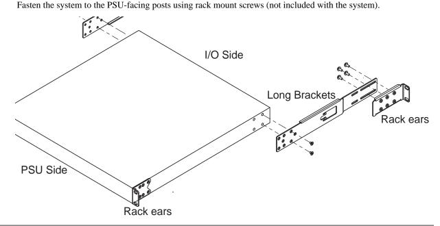
Use the provided pan head screws to attach the rack ears on the I/O-facing posts to the long bracket previously attached to the system. Tighten the pan head screws to secure the system.
